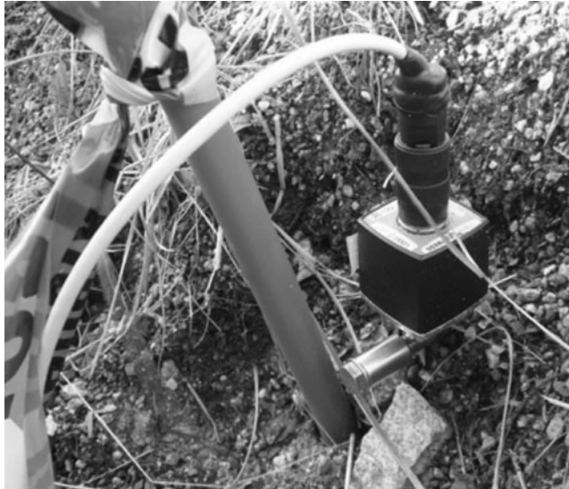
Figure 1 The sensor was mounted on a metal bar that penetrated approximately 1 m horizontally into the ground about 0.3 m below the paved road surface. In this image, the pavement extended from the upper right corner. Visible are the sensor, the left end of the metal bar, the Ethernet cable, and a roadside marker that located the sensor in the environment.
